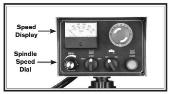
Figure 35. Spindle speed dial and display.
